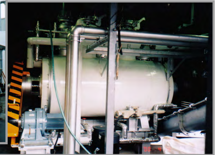
KVD-20Y (vegetable residue processing 3t/per day)
